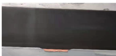
图 11 安全充电方法循环后的负极极片 Fig.11 Negative pole piece after cycling by safe charging method
