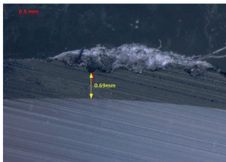
图 2 外半导电层显微镜下放电痕迹 Fig.2 Discharge traces of fault cable outside semiconducting layer in microscope
