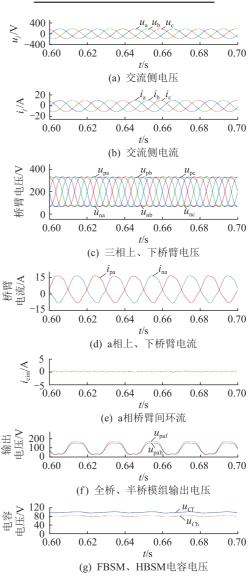
图 11 优化控制策略下的混合型 MMC 稳态运行波形 Fig.11 Steady-state operation waveforms of hybrid MMC under optimized control strategy
