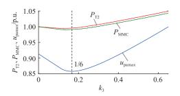
图 4 三次谐波电压注入对损耗的影响 Fig.4 Influence of third harmonic voltage injection on loss
