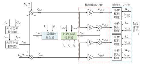
图 8 基于三次谐波电压注入及桥臂输出电压差异化分配的混合型 MMC 控制框图 Fig.8 Hybrid MMC control block diagram based on third harmonic voltage injection and arm output voltage differential distribution
