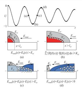
图 14 振动冲击激励下绝缘子沿面局部放电形成机制 Fig.14 Propagations of discharge along the insulator surface with varying background electric field
