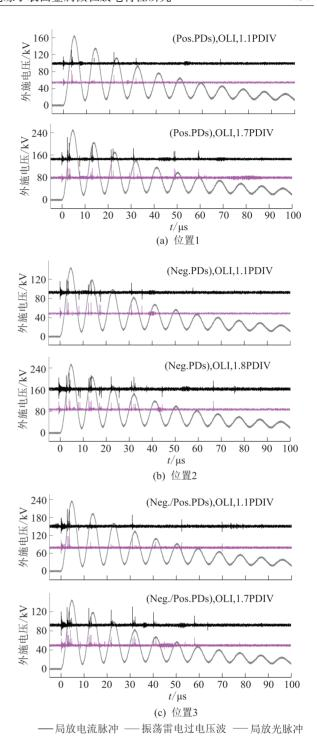
图 9 OLI 电压下电流脉冲和光脉冲 Fig.9 PD current and light sequences under OLI particle at position
