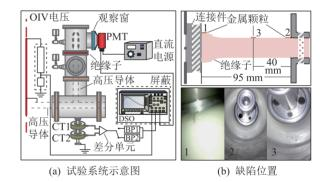
图 6 测试系统及人工缺陷放置位置 Fig.6 Test system and placement of artifical defects
