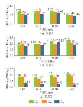
图 8 不同电压下 3 种外施电压的激发系数 Fig.8 Efficiency factors of OLI, OSI, and AC voltages at various gas pressures
