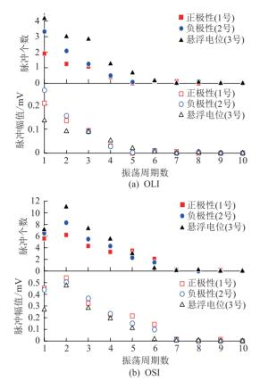
图 12 前 10 个周期下局部放电脉冲数及其幅值 Fig.12 PD numbers and PD magnitudes in the first ten oscillating periods
