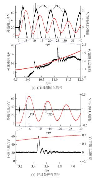
图 4 限制前后的电容性位移电流及局部放电信号 Fig.4 Signals before and after processing output signal of CT1 and processed PD signal
