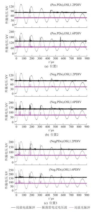
图 10 OSI 电压下电流脉冲和光脉冲 Fig.10 PD current and light sequences under OSI particle at position
